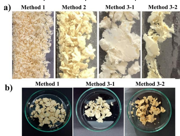
Figure 3. Three different procedures for extracting cellulose from SS4. a) The SSC in the SS4 form applied to different experimental procedures, b) The RHC in the form of the RH1 subjected to different experimental procedures.
