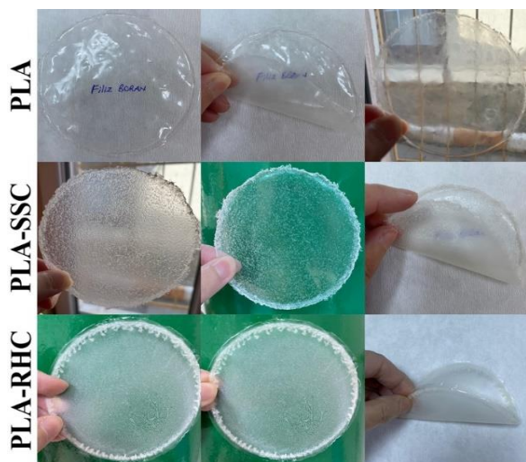
Figure 5. Digital images of cellulose-reinforced PLA bioplastic films.
