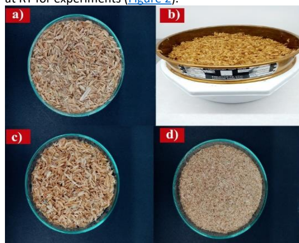
Figure 2. RH Pre-treatment. a) The RH sample, b, c) the sieving and washing process, d) the ground RH1 sample.
