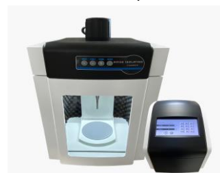
Figure 2. Ultrasonic-assisted extraction device used to obtain the terebinthus fruit extracts.
