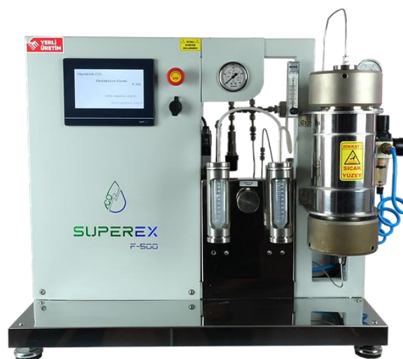
Figure 1. Supercritical CO 2 extraction device used to obtain the terebinthus fruit extracts.
